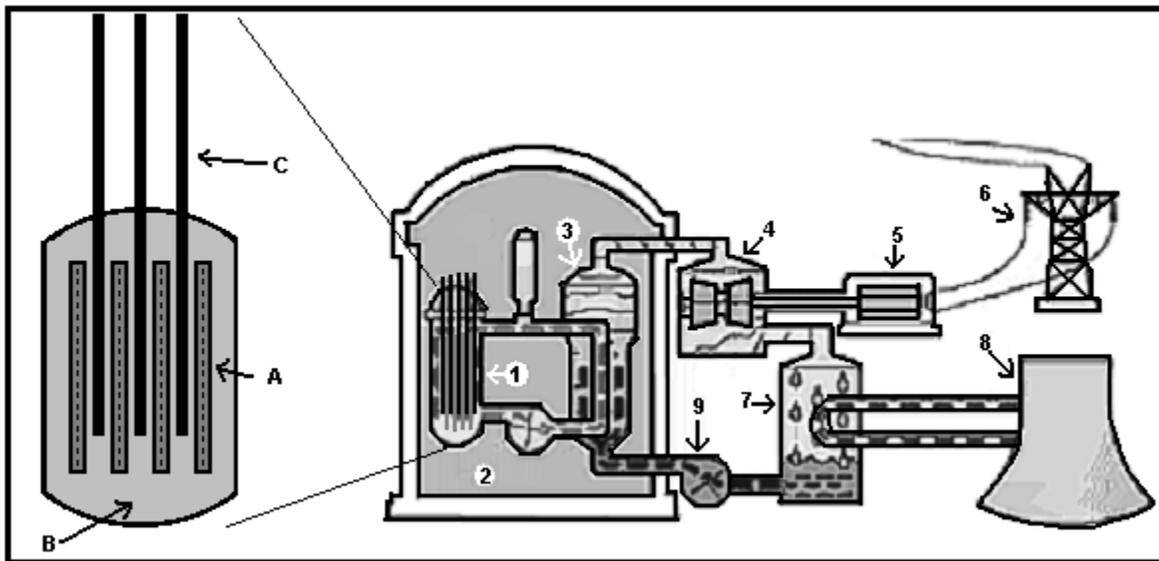
The process by which a nuclear reactor converts the heat released by a nuclear fission reaction into electricity.
